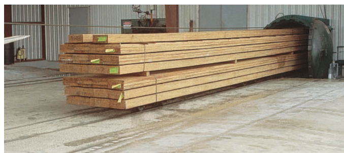
Parallam® PSL products enter an airtight treatment cylinder—a highly controlled, pressurized environment where they are exposed to the treatment process.
