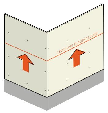
Start at the bottom of one end of the wall with the side without fiber facing up. When starting at a corner, overlap by a minimum of 6" (152 mm). A minimum of a 1" (25.4 mm) overlap on the sill plate is required; however, for maximum protection, a 2"-4" (51–102 mm) overlap on the sill plate is recommended.
